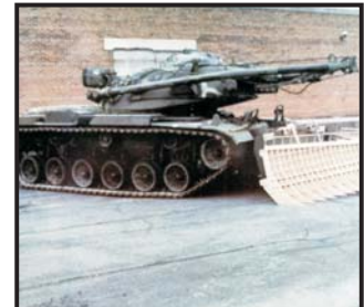
Mine rakes are manufactured to clear large areas of mines during the Gulf War.
